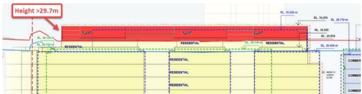
Figure 47: Building C - Wattle Street Section Detail: Height >29.7m (Sydney LEP 2012, clause 6.21D)
