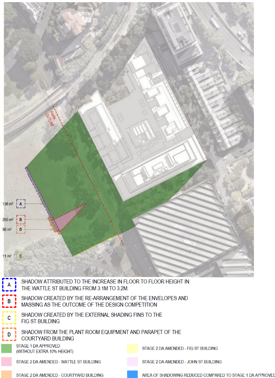
Figure 48: Building D - Wattle Street, Building C - Courtyard and Building E - Fig Street: Shadow diagram at 9am in midwinter
